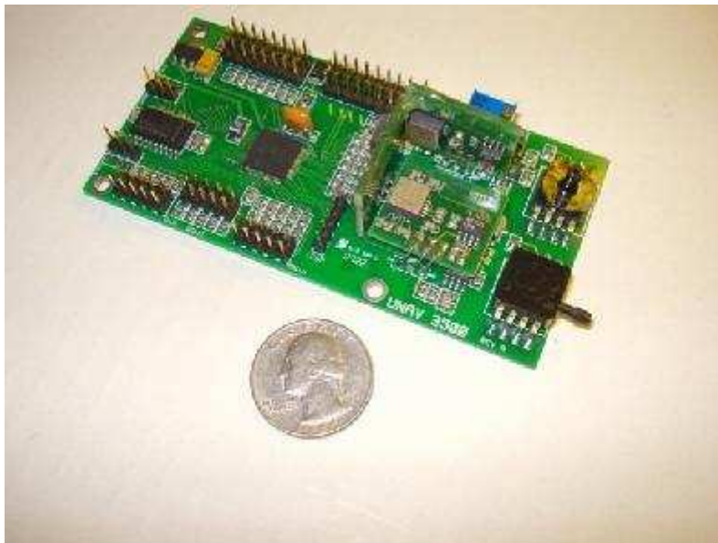
UNAV3500 Series Autopilot Board (By UNAV-LLC)
